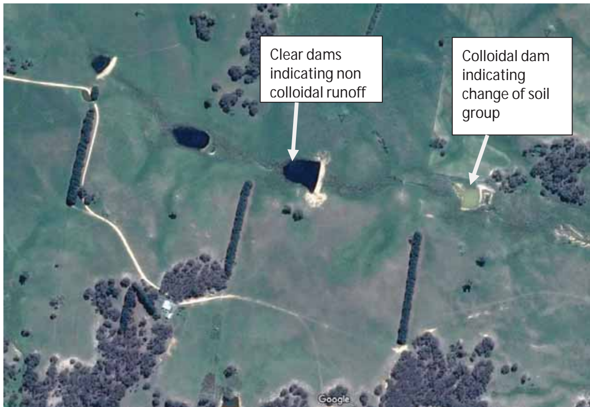
Plate 3 showing the site with three easterly dams with clear water and the westerly dam with colloidal water (image courtesy Google Earth Pro)
